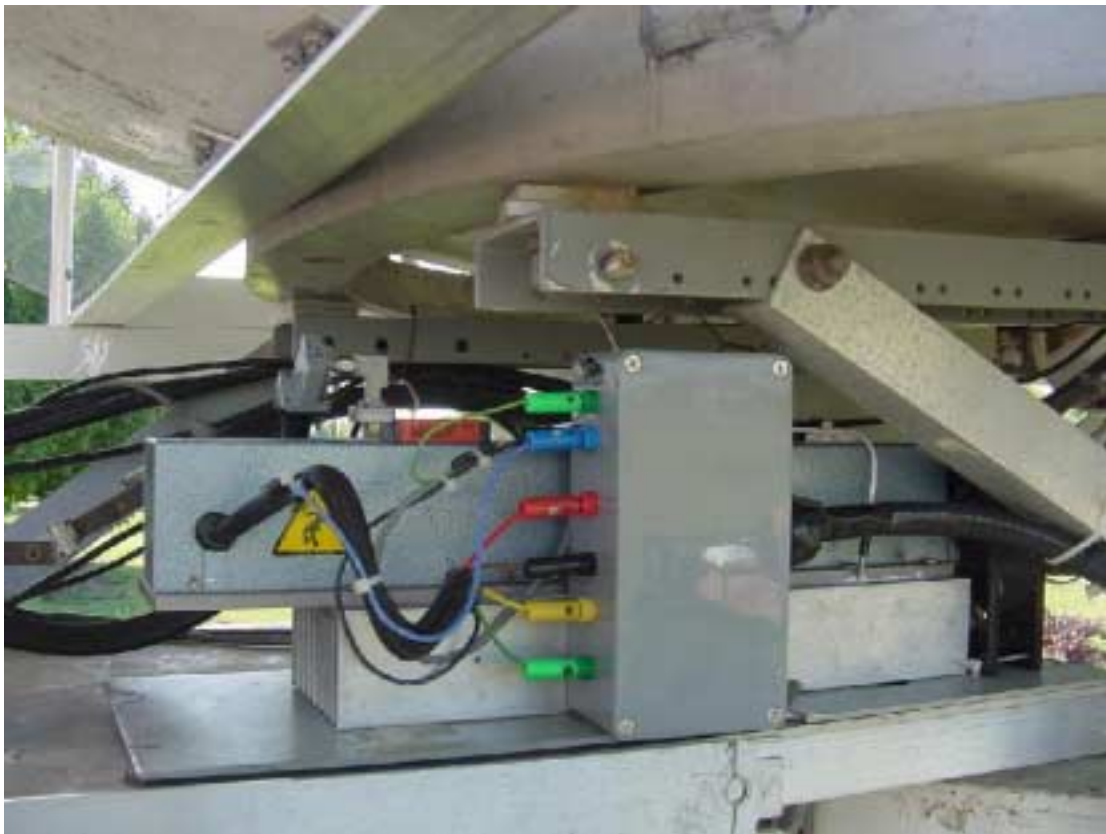
Figure 11 TH-3864C TWT Mounted behind dish. Note high voltage junction box and magnet.
