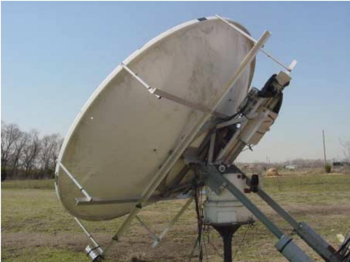
Figure 5. Back structure for 3 Meter Dish at W5LUA
